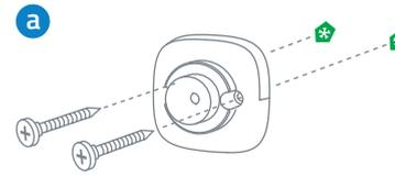
Drill holes with a **15/64 in (6 mm)** drill bit, then insert the anchors into the holes; anchors are necessary for walls that are made out of hard materials such as concrete, brick, or stucco.
