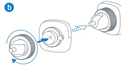
Screw the base of the outdoor mount onto the wall. Fasten the ball bracket of the outdoor mount to the base of the outdoor mount.
