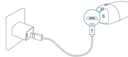
Use the provided micro-USB charging cable to connect eufyCam to the camera charging port on the backside of the HomeBase. Charging a camera takes approximately 4 hours; it will take longer if you charge the camera via a universal 5V USB charger.
