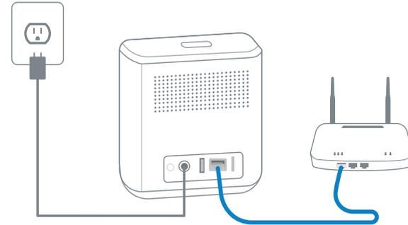
2. The LED indicator turns to white (this may take up to 1min) when HomeBase is ready for setup.
