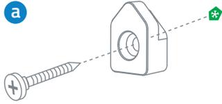
Drill a hole. Use the included anchor if it's drywall and fasten the hook.
